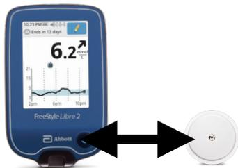
For the alarm to work, the reader needs to be within 6 metres of the sensor.
